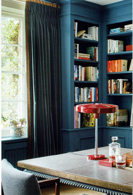
ABOVE This wood-paneled library was designed by Artichoke and made from European walnut by the company's craftsmen at its workshop in Somerset. The panelling was finished by hand with French polish.
