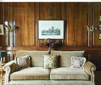
ABOVE This wood-paneled library was designed by Artichoke and made from European walnut by the company's craftsmen at its workshop in Somerset. The panelling was finished by hand with French polish.
